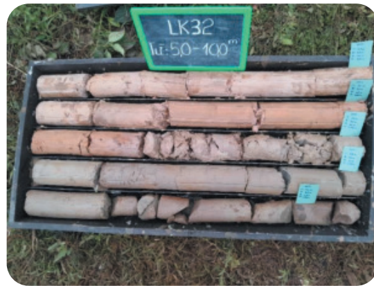
Photo. Drilling operations and diatomite drill core samples in the An Xuan area
