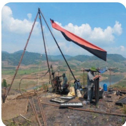
Photo. Drilling operations and metacarbonate drill core samples in the Kon Roi area, KBang Commune, Gia Lai Province
