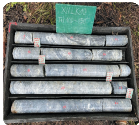
Photo. Drilling operations and metacarbonate drill core samples in the Kon Roi area, KBang Commune, Gia Lai Province
